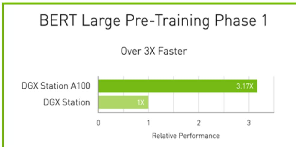
Figure 18. BERT Large Pre-Training, Speedup of DGX Station A100 relative to DGX Station. Batch Size=64; Mixed Precision; With AMP; Real Data; Sequence Length=128
