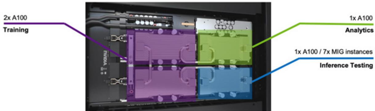
Figure 8. Different workloads on different GPUs in NVIDIA DGX Station A100 system.
