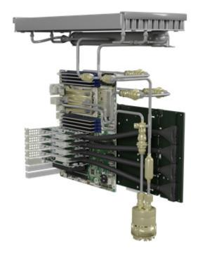
Figure 12. Figure 10. View of NVIDIA DGX Station A100 cooling system.
