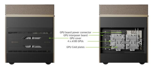
Figure 10. View of NVIDIA DGX Station A100, GPU side, with GPU cold plates.
