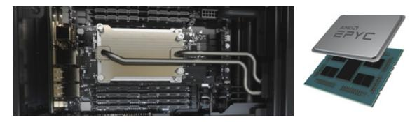
*Figure 13. View of the AMD Epyc 7742 processor, covered by its cold plate.*
