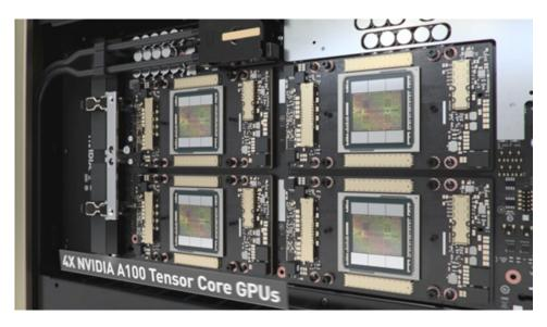
Figure 9. View of the 4-way NVIDIA HGX board inside NVIDIA DGX Station A100.
