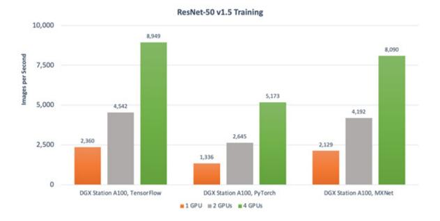
*Figure 20.* DGX Station A100 (4x A100 SXM 80GB), ResNet-50 V1.5 training, Mixed Precision, TensorFlow (21.02-tf1\_py3, bs 256), PyTorch (21.02\_py3, bs 256), MXNet (21.02\_py3, bs 192)
